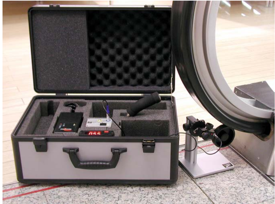
Miniwheel 80 with P110 display measuring speed on an escalator handrail
